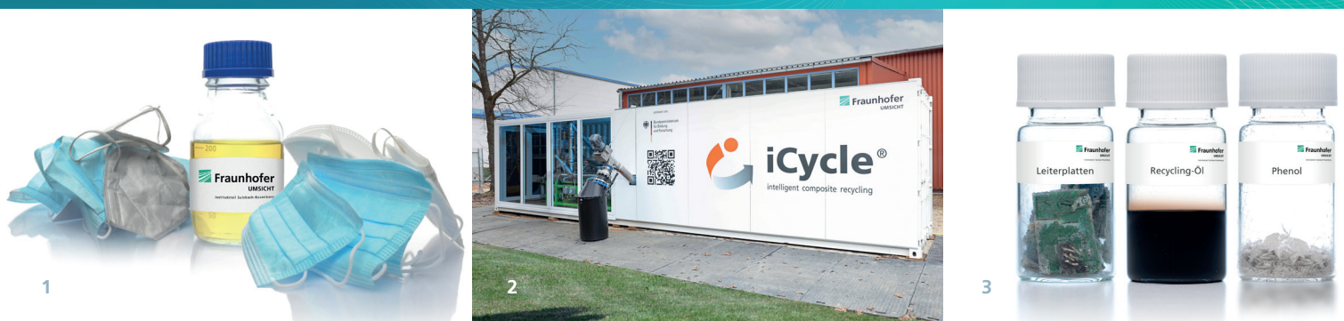
1 Closed loop recycling: mouth-nose-protection 2 Continuous pyrolysis plant (iCycle®70) 3 Electronic scrap (feedstock), pyrolysis oil (intermediate), and phenol (product)
